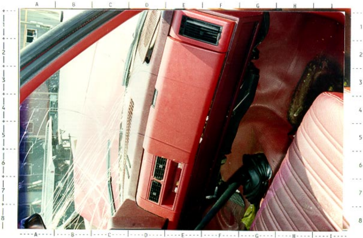
# 89 -- Front center & right dash areas of 1988 Chevrolet pickup; NOTE: undamaged dash and minor intrusion to toepan area
